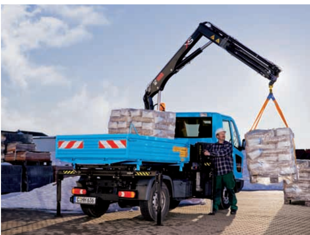
Customers can choose to operate the cranes by remote or manually by the levers. These are placed vertically to provide more room for the load.
